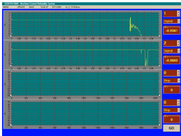
Figure 2: Time waveform Channels 1 & 2 during shear impacting. This graph illustrates that vibration resulting from the shears are much greater than steady-state vibrations. It illustrates how channel 1 "ring" for several seconds transmitting large amounts of vibration energy to the structure shoe plate and subsequently the foundation (see Channel #2). Although channel #2 does not "ring" like channel #1, the vibration energy is transmitted to the foundation.
